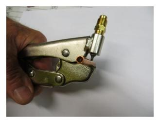
Screw the valve back into the piercing plier.
