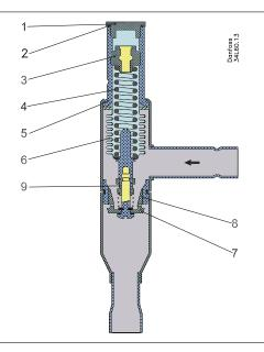
Hot gas bypass regulator type KVC opens on a fall in pressure on the outlet side, i.e. when the pressure in the evaporator reaches the set value.
