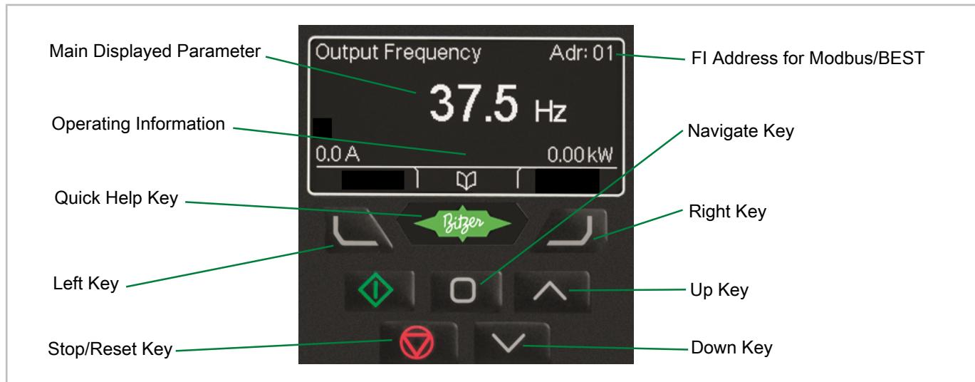
**Main Displayed Parameter:** Shows which of the selectable parameters is currently being shown on the main display, e.g. motor speed, motor current etc.
