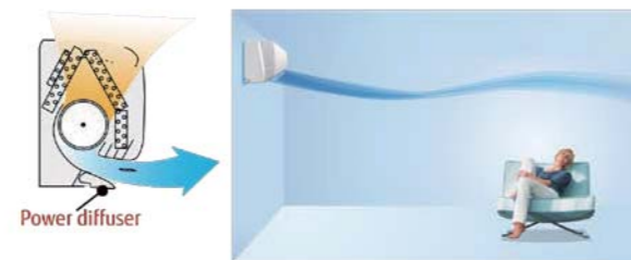
Horizontal airflow does not blow cool air directly at the occupants in the room.
